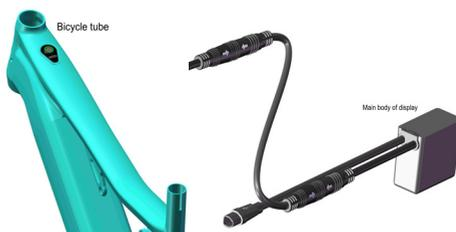
3. Dock the DP's male connector "h" with EB-BUS's female connector "H" as indicated.
